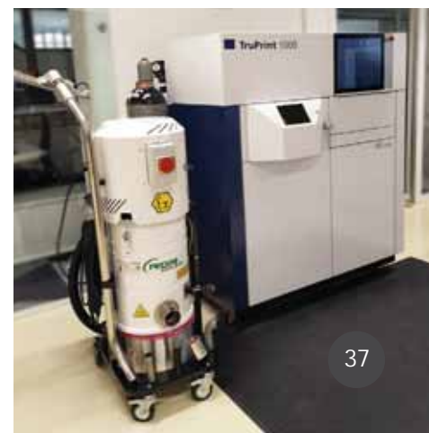
Tank with liquid abatement system to inertising reactive dust
